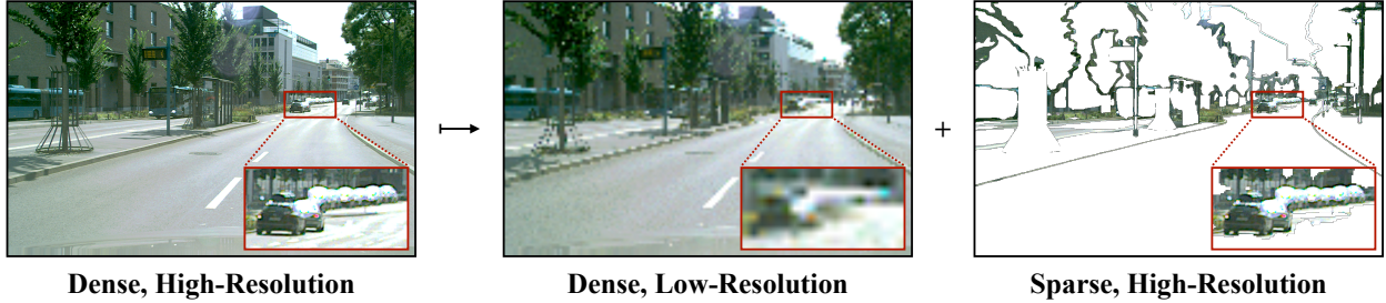
Figure 2.6: Processing dense high-resolution inputs is computationally expensive. We propose an alternative approach by integrating dense low-resolution and sparse high-resolution inputs, which provide complementary information about the overall scene layout and intricate object details. Leveraging the lower resolution and sparsity of these inputs allows for more efficient processing.
